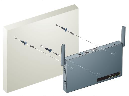
FIGURE 2-4 Hanging the Aruba 52 on Screws
