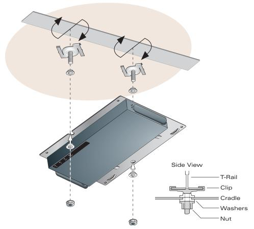
FIGURE 2-7 Mounting on a Suspended Ceiling
