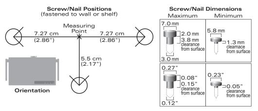
FIGURE 2-3 Mounting Screw Specifications
