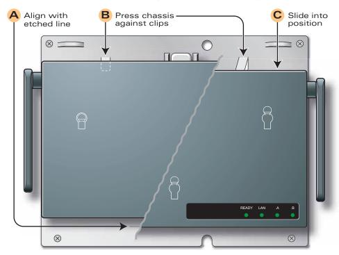
FIGURE 2-6 Placing the Aruba 52 into the Cradle
