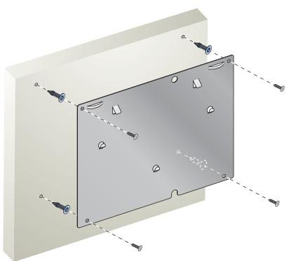
FIGURE 2-5 Attaching the Mounting Cradle
