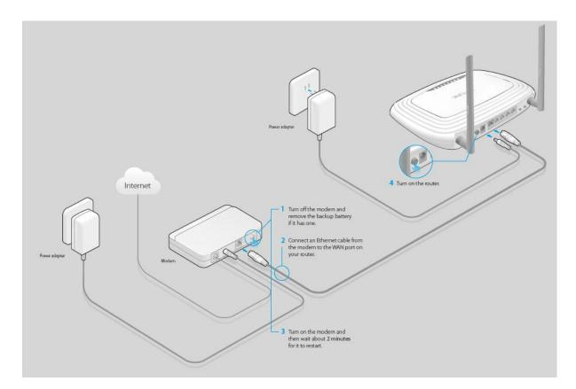
Figure 2-1 Hardware Installation
