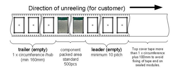
Empty spaces in the component packed area shall be less than two per reel and those spaces shall not be consecutive.
