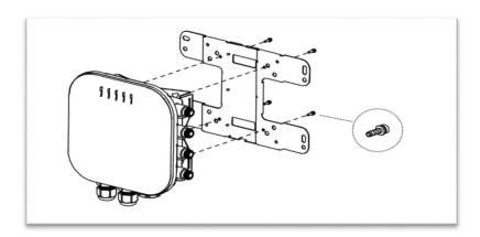
4) Attach the device on to the wall by tightening the bolt's flat washer and nuts to secure the mounting base to the mounting surface.
