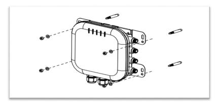
**Note:** The installation is correct if the node does not easily move from side to side. **Best practice:** Use a spray to prevent corrosion on the bracket and mount hardware.
