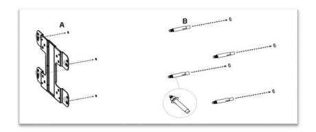
3) Place the lock and flat washer on the four hex cap screws and drive the screws to attach the bracket to the back of the Mesh node.
