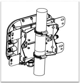
**Note:** The installation is correct if the node does not easily move from side to side. **Best practice:** Use a spray to prevent corrosion on the bracket and mount hardware.
