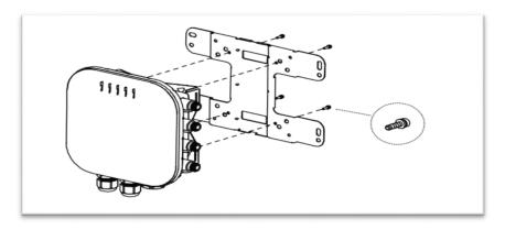
2. Drive the four round head screws to attach the pole mount bracket to the wall mount bracket.
