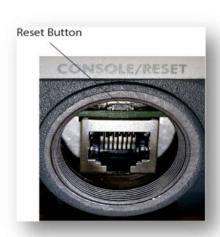
Reset button is above the console port RJ45 connector.
