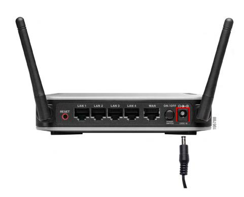
**STEP 5** Plug the other end of the adapter into an electrical outlet.
