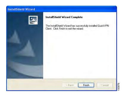
STEP 3 Click Finished to complete the installation. Proceed to "Using the Cisco QuickVPN Software," on page 142.
