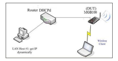
**Wireless Client Mode:** First, please configure the wireless setting of MGB100 via wire. Then use Scan AP of AP-List and join it. Plug up the cable form MGB100. The client from LAN can use "Configure" utility to Query.
