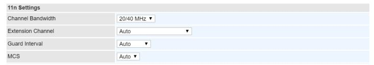
**Channel Bandwidth:** Select **20 MHz, 40 MHz,** or **20/40 MHz** for the channel bandwidth. The wider the Channel bandwidth the better the performance will be.
