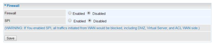
**Firewall:** To automatically detect and block Denial of Service (DoS) attacks, such as Ping of Death, SYN Flood, Port Scan and Land Attack.
