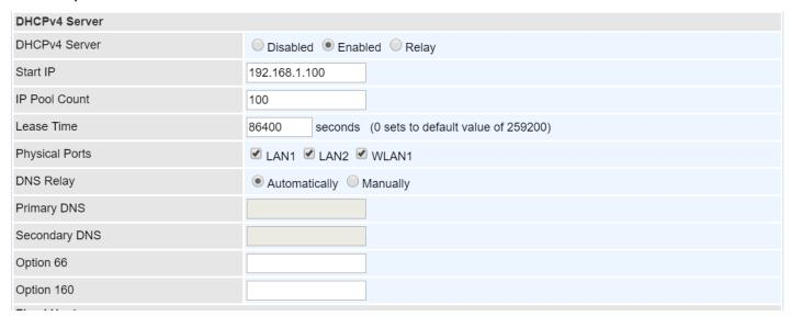
**DHCPv4 Server:** If set to **Enabled**, your MX-210NPV can assign IP addresses, default gateway and DNS servers to the DHCP client.
