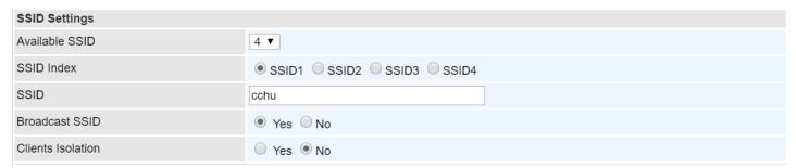
Available SSID: User can determine how many virtual SSIDs to be used. Default is 1, maximum is 4.
