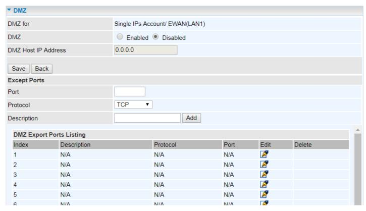
**DMZ for (via a WAN Interface):** Allows outside network to connect in and communicate with internal LAN devices via a specific WAN interface.
