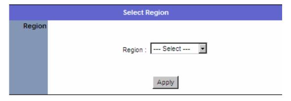
**Warning:** This device requires that the user or installer properly selects the current region of operation before using this device. This device will automatically limit the allowable channels determined by the current region of operation.
