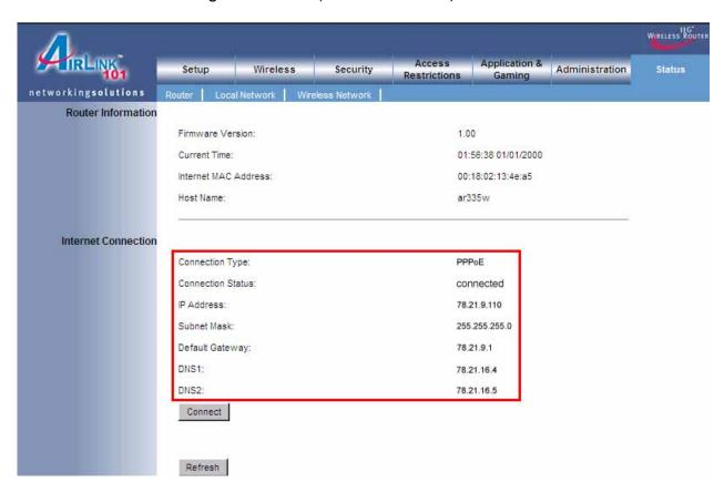
If each field has a valid number assigned, the router is connected to the Internet.
