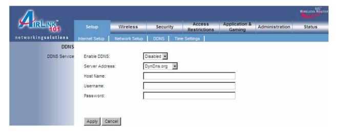
To Enable DDNS, select the DDNS provider you have registered with and enter the required fields. Click **Apply** and **OK** to save the setting.
