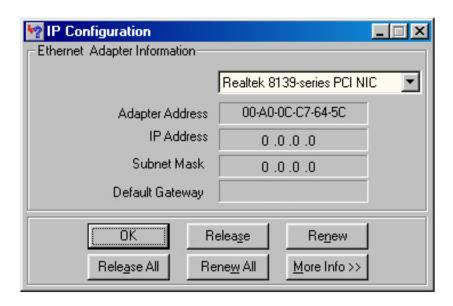
**Step 8** After your IP address is released, click **Renew**. You should get an IP address of **192.168.1.x** (where **x** is a number between 2 - 254). If you don't get an IP address, reset the router by holding in the reset button on the back of the router for 10 seconds while it is ON and try **Renew** again.
