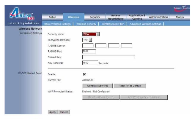
**Encryption Methods**: Select either **TKIP** or **AES** as the encryption method.
