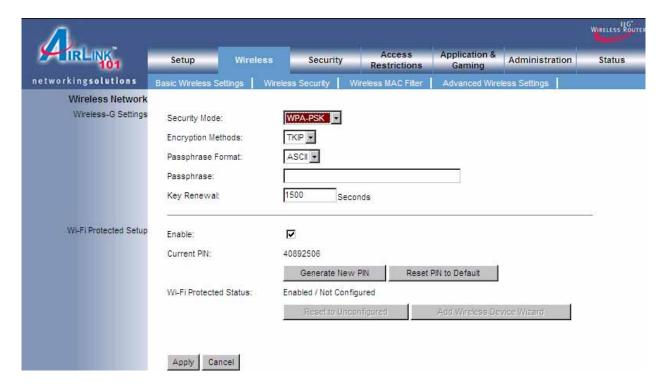
**Encryption Methods**: Select either **TKIP** or **AES** as the encryption method.
