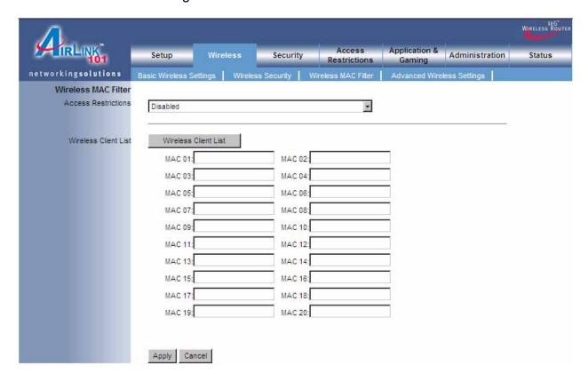
Select **Enabled** from the drop-down menu and choose whether the specified wireless clients will be prevented or permitted to access the wireless network. Enter their MAC address in the fields below and click **Apply** and **OK** to save the settings.
