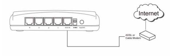
2. Connect all your computers, network devices (network-enabled consumer devices other than computers, like game console, or switch / hub) to the LAN port of the router.
