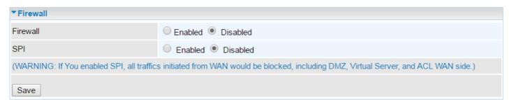
**Firewall:** To automatically detect and block Denial of Service (DoS) attacks, such as Ping of Death, SYN Flood, Port Scan and Land Attack.
