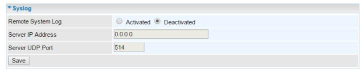
Remote System Log: Select Activated to enable this feature
