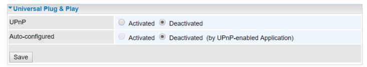
**UPnP:** Select this checkbox to activate UPnP. Be aware that anyone could use an UPnP application to open the web configuration's login screen without entering the MX-230 M1's IP address
