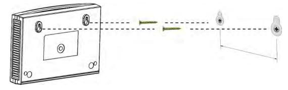
Figure 2 Wall Mounting Example
