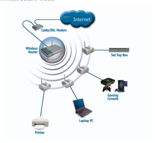
This example illustrates an **Infrastructure** setup. To connect the DWL-G810 to a wireless network with a wireless router or access point, please refer to the printed Quick Installation Guide included with the product. Web configuration is required to connect the DWL-G810.
