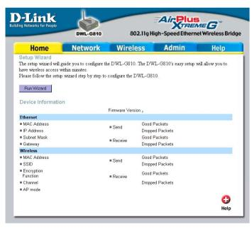
This window displays the default settings of the DWL-G810. The default IP address is 192.168.30. If you select **Dynamic IP Address**, you will obtain a dynamic IP address from a DHCP server on your network.
