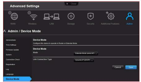
4. To configure LAN Connection Type, select Dynamic IP (DHCP) (default) or Static IP, complete the required fields, and click Save. (See "" on page 46 for details.) the screen informs you of how long the process will take. The router reboots, and the login screen displays.
