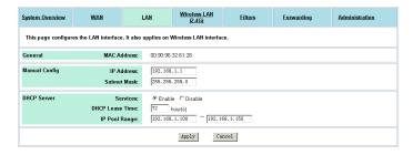
Figure 4-8 LAN Configuration in Router Mode
