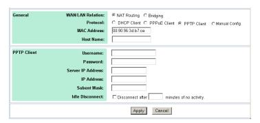
Figure 4-6 WAN Configuration-PPTP Client
