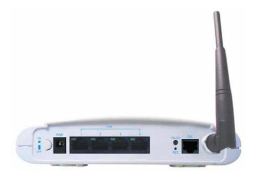
Figure 3: X7968r Rear Panel Connections
