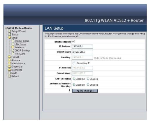
**IP** Address: This is the IP address of the router. The default IP address is 192.168.1.1.
