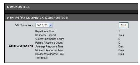
To start the test, select the **DSL Interface** from the drop-down list, and then click the **Test** button.
