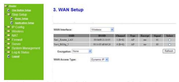
The Wireless network which searched by Server Router will display on this page. Users can select the desired wireless network and Encryption type to connect.
