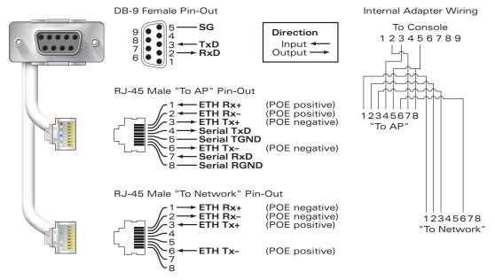
FIGURE A-2 Aruba Serial Breakout Adapter
