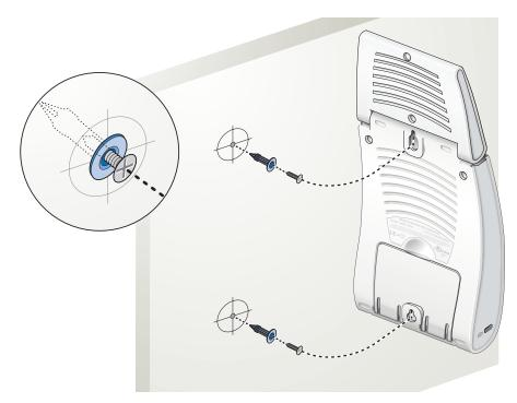
FIGURE 3-4 Hanging the Aruba 60/61 on Screws
