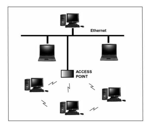
Figure 3 Infrastructure Mode-Combination Wireless and Hardwired LANs
