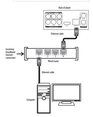
2 Connect an Ethernet cable (CAT5 or better with RJ45 connector) to the router and the computer.
