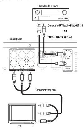
2 Connect a digital optical cable to the OPTICAL DIGITAL OUT jack on the back of your TV and to the OPTICAL DIGITAL IN jack on the receiver. Or
