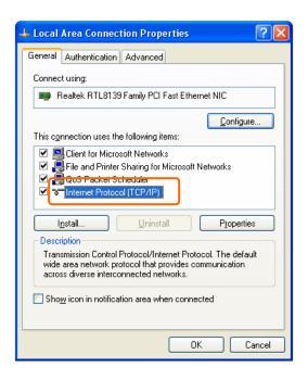
**Step 4-1.** For getting IP automatically if you are one of the users under 11N Broadband router, please skip **Use the following IP address** and then select **Obtain an IP address automatically** and **Obtain DNS server address automatically** and then click on **OK** button.
