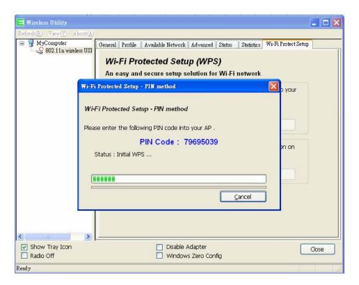
(2.) Open menu "Wi-Fi Protected Setup" of 11N Broadband router, input the PIN number from the wireless card then click Start PIN.
