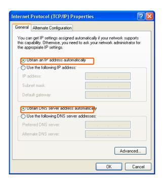
**Step 4-2.** For getting IP manually in order to specify a Virtual Server, such as Print Server, FTP Server and so on, please skip **Obtain an IP address automatically** and then select **Use the following IP address**. And the following default setting of 11N Broadband router should be noted:
