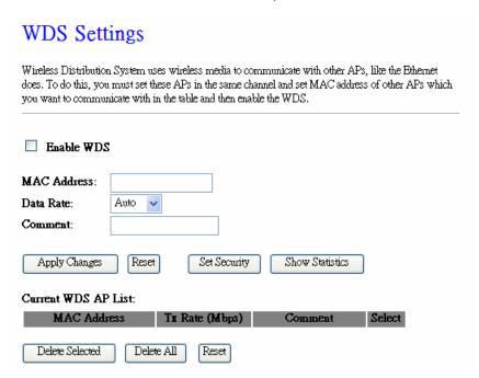
**Step 1.** Check the MAC address and Channel number of the device you want to setup WDS with 11N Broadband router.
