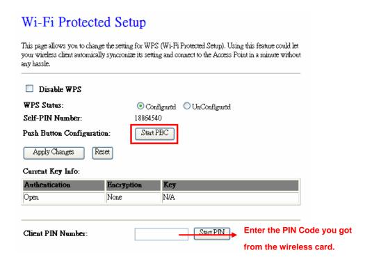
(3.) Back to "Wireless Utility" and press the "Start PIN" button to complete the auto-paring process.
