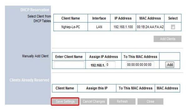
**Step 1** Enter the Static IP Address in the **Assign this IP** field.
