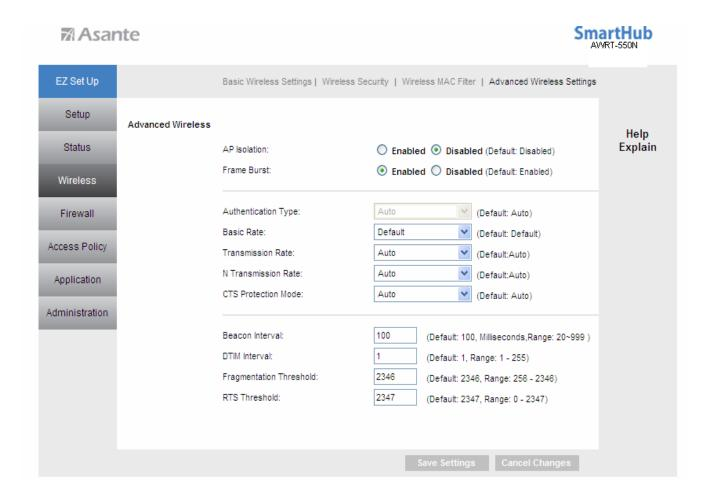
**AP Isolation:** This isolates all wireless clients and wireless devices on your network from each other. Wireless devices will be able to communicate with the Router but not with each other. To use this function, select **Enabled**.
