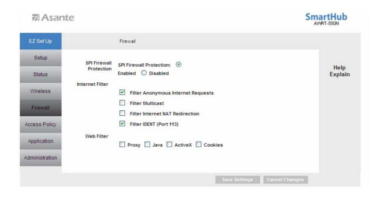
**SPI Firewall Protection**: Select to enable or disable Stateful Packet Inspection. When enabled, access to the router from internet/wan by various protocols like ICMP are denied.
