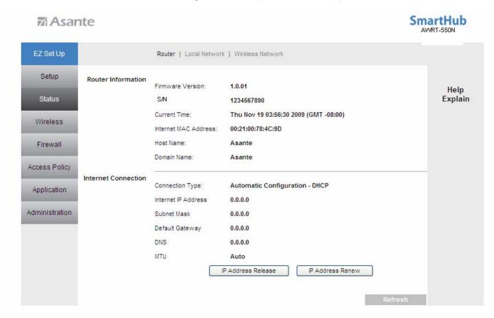
If each field has a valid numbers(not all 0's) assigned, the router is connected to the Internet.
