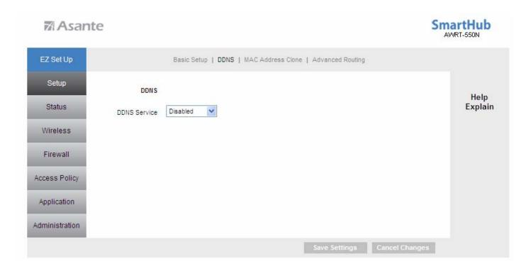
To Enable DDNS, select the DDNS provider you have registered with and enter the required fields. Click **Save Settings** to save the settings.
