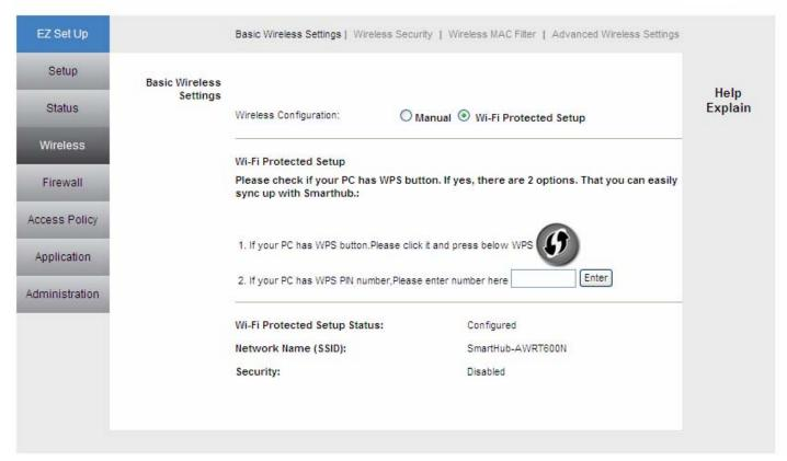
WiFi Protected Setup supports two types of connection: Push Button Configuration (PBC) or Personal Identification Number (PIN).
