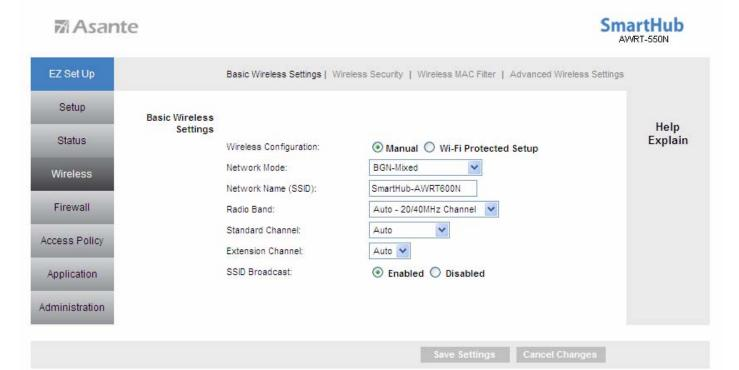
**Network Mode**: If you have 802.11b/g/n 2.4GHz devices on the wireless network, select **BGN-Mixed**. If you have 802.11a/n 5GHz devices on the wireless network, select **AN-Mixed**.
