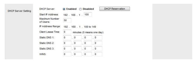
**Start IP Address:** Give a value for the dynamically assigning IP address to start with. Because the Router's default IP address is **192.168.1.1**, the Starting IP Address must be 192.168.1.2 or greater, but smaller than 192.168.1.253. The default Starting IP Address is **192.168.1.100**.
