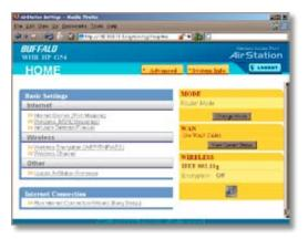
This is the opening page of your AirStation's configuration tool. You can always get to it from within the configuration screens by clicking on *Home*. From here, you can configure port mapping for your internet games, turn on UPnP for Windows (MSN) Messenger, configure your Firewall, setup Encryption, choose your Wireless channel, update your AirStation's firmware, and reset your Internet connection's configuration. As you explore the configuration tool, you can
