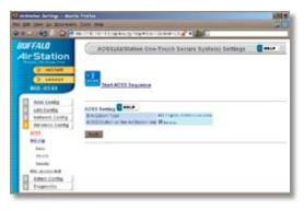
Clicking *Start AOSS Sequence* has the same function as pushing the AOSS button on the router: it initiates the AOSS process.
