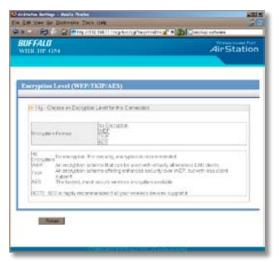
This page is available from *Home* by selecting *Wireless Encryption*. Here, you can manually select the type of wireless encryption you'd like to use. Your AirStation supports three different encryption schemes; choose the best one that all your clients support.
