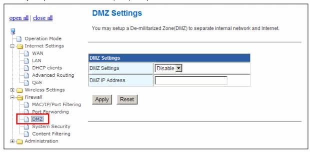
**DMZ Setting:** If the DMZ Host Function is enabled, it means that you set up DMZ host at a particular computer to be exposed to the Internet so that some applications/software, especially Internet/Online game can have two-way connections. Select Enable or Disable from the pull-down menu.
