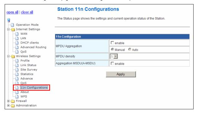
**MPDU Aggregation:** MPDU stands for MAC Protocol Data Unit. MPDUs are the fragmented units of MSDU, also called MAC frames, encapsulate the higher layer protocol data or contain MAC management messages.
