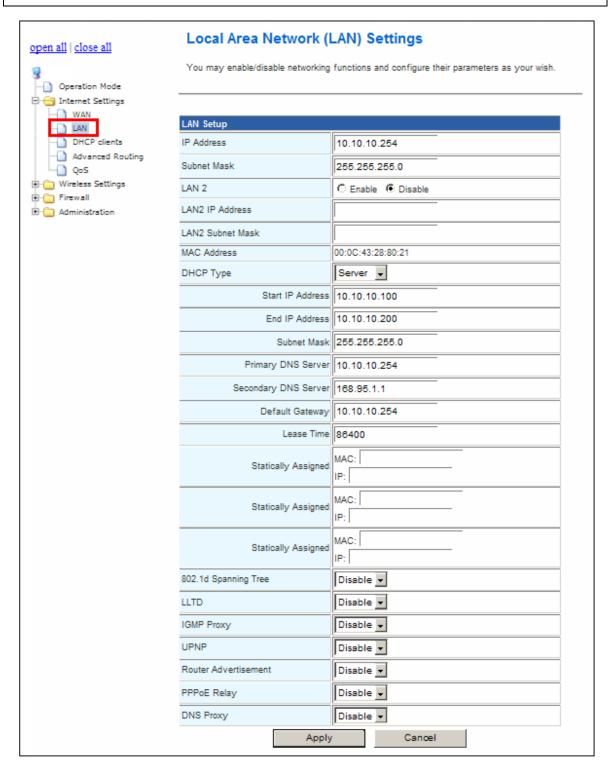
LAN IP Address: The LAN IP address. Default: 192.168.1.1 Subnet Mask: The LAN net-mask. Default: 255.255.255.0
