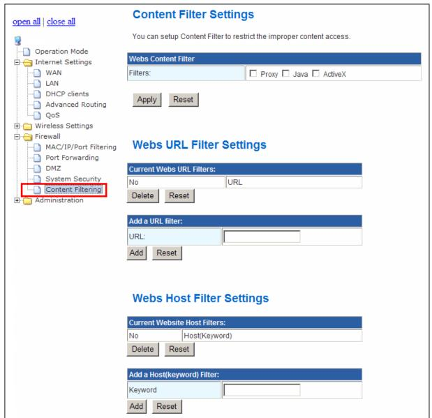
**Content Filter Setting:** There have three options for this filter – Proxy, Java, and ActiveX.When those options are checked, the content filter will deny computer from access to the internet by contented those options.
