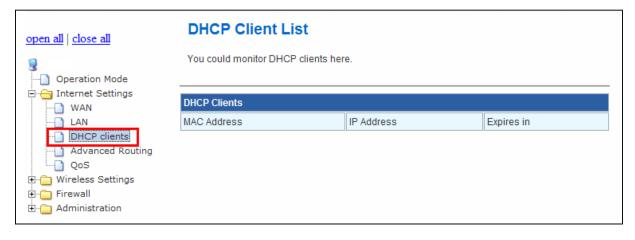
**MAC Address:** Shows the client MAC address information. **IP address:** Shows the client IP address information. **Expires in:** Shows the expired time of the client.
