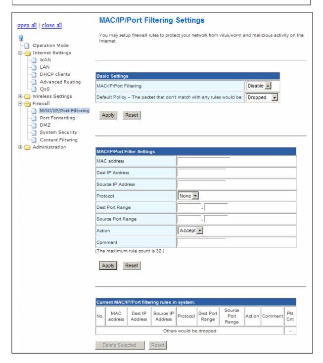
**MAC/IP/Port Filtering:** Enable this function, all list from the filtering will be deny the internet
