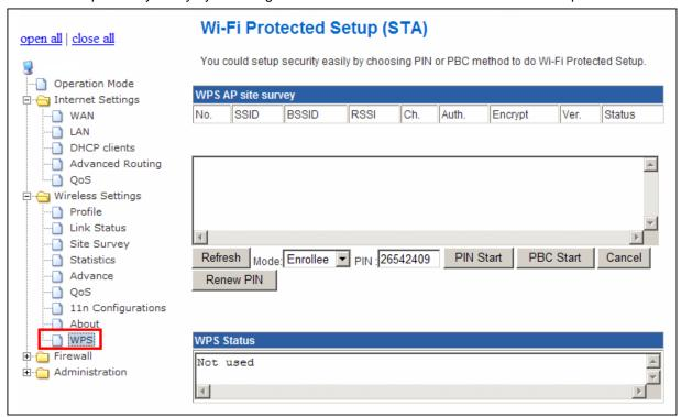
**WPS AP Site Survey:** Display the information of surrounding APs with WPS IE from last scan result. List information includes SSID, BSSID, RSSI, Channel, ID (Device Password ID), Auth., Encrypt, Ver., and Status.
