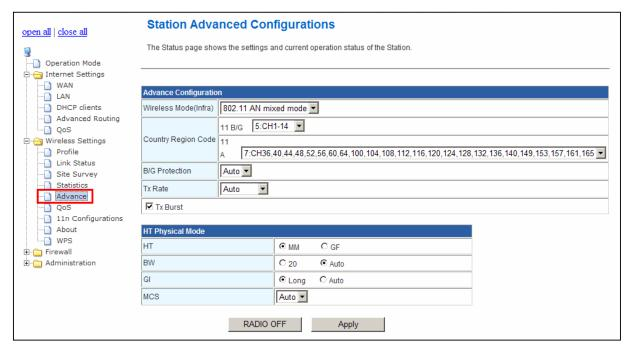
**Wireless Mode:** Select wireless mode. 802.11A Only, 802.11 AN mix mode are supported. **Country Region Code:** This field displays the region of operation for which the wireless interface is intended.
