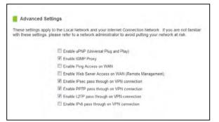
media, such as an Ethernet connection or wireless connection. With UPnP enabled, network devices may change security settings within the Router's firewall to allow access over the Internet. By default, UPnP is disabled to avoid exposing your network to security issues.
