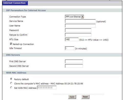
Figure 51 Network > WAN > Internet Connection: PPPoE Encapsulation
