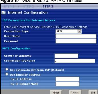
Figure 19 Wizard Step 3: PPTP Connection
