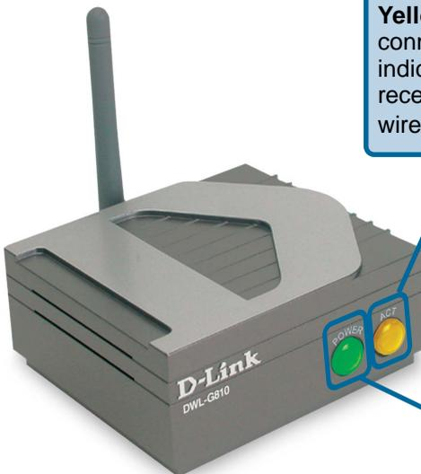
**Wireless Link/Act** – a steady **Yellow** light indicates a wireless connection. A blinking light indicates that the DWL-G810 is receiving/transmitting from/to the wireless network.
