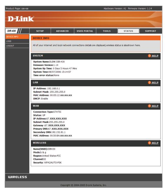
As shown above, the welcome page represents the status of the various parameters of the DIR-430. The Top pane shown in the figure provides the sections of the DIR-430 configuration. The left pane shown in the figure provides the relevant sub-sections of DIR-430 configuration. Each section gets expanded when clicked to show few hyperlinks. Each hyperlink allows you to configure certain parameters of the Gateway.
