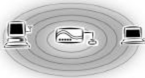
Figure 1. Simple Wireless Infrastructure Network
