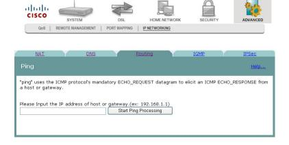
5 Enter the IP address of a remote host and click **Start Ping Processing**. The Ping result appears on the screen as shown below.
