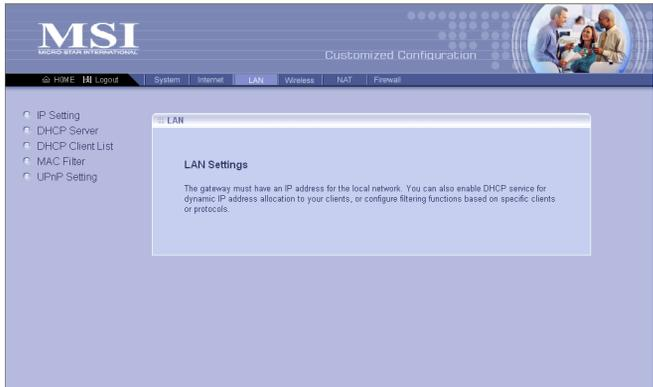
\* The default IP Address for the LAN Port is 192.168.1.254; and for DMZ port is 192.168.2.254. See Appendix B for details.
