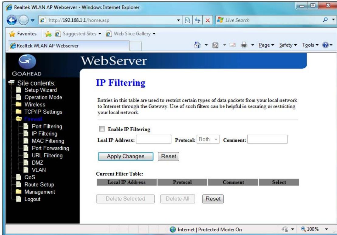
**Enable IP Filtering:** Click to enable the IP filtering security function.
