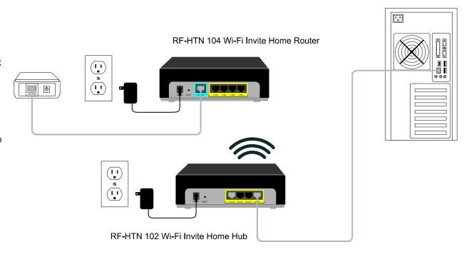
5. When you have completed the setup, move the hub to desired location and connect the power adapter. Connect the devices you want to use into the DEVICE ports on the back of the hub.
