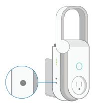
The Reset button is located on the left side of the Wi-Fi Extender+.
