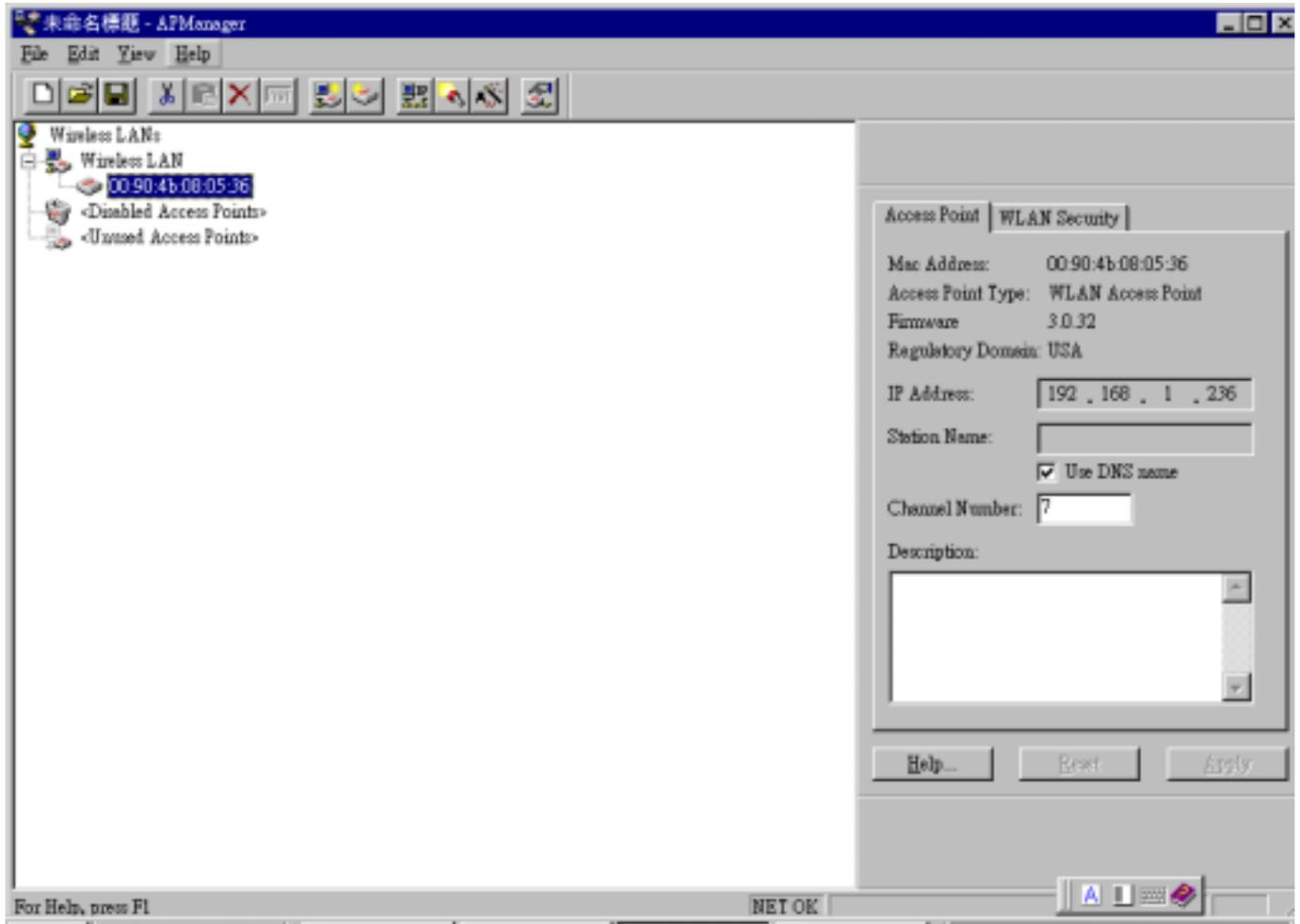
The tree structure on the left of the window shows a list of WLANs (Wireless LANs) and the Access Points that are part of each WLAN. The sample image above shows a single Access Point with hardware address 00:90:4b:08:05:36 that is assigned to the WLAN named "Wireless LAN". The icons indicate the status of the WLANs and their associated Access Points.
