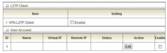
Enable VPN-L2TP Client, and press "Edit" button to add connection detail.
