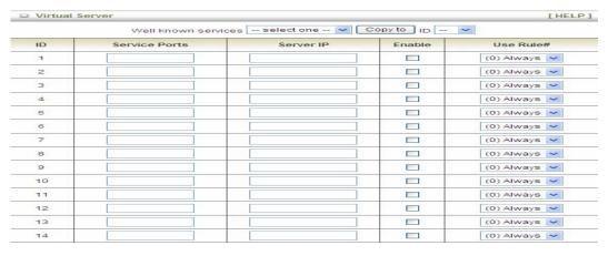
For example, if you have an FTP server (port 21) at 192.168.123.1, a Web server (port 80) at 192.168.123.2, and a VPN server at 192.168.123.6, then you need to specify the following virtual server mapping table:
