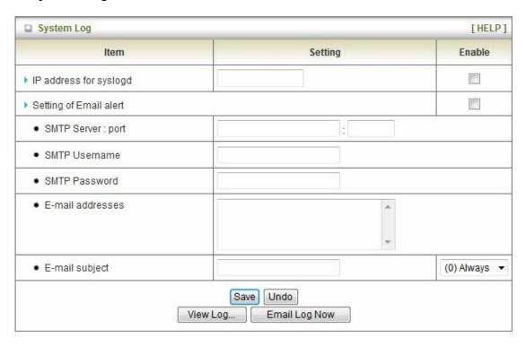
This page support two methods to export system logs to specific destination by means of syslog (UDP) and SMTP(TCP). The items you have to setup including:
