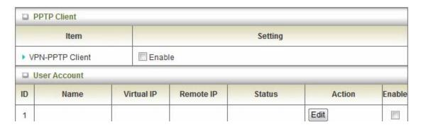
Enable VPN-PPTP Client, and press "Edit" button to add connection detail.
