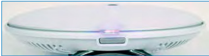
Figure 4: Purple LED – Booster is syncing
