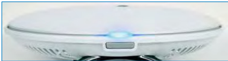
Figure 5: Blue LED – sync is complete
