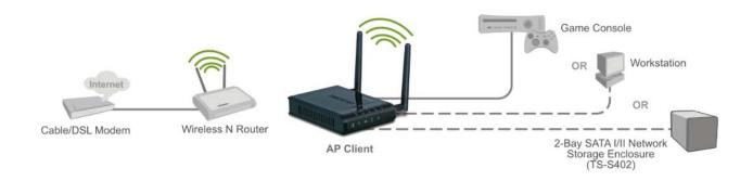
AP Client allows Ethernet enabled devices to become wirelessly enabled.
