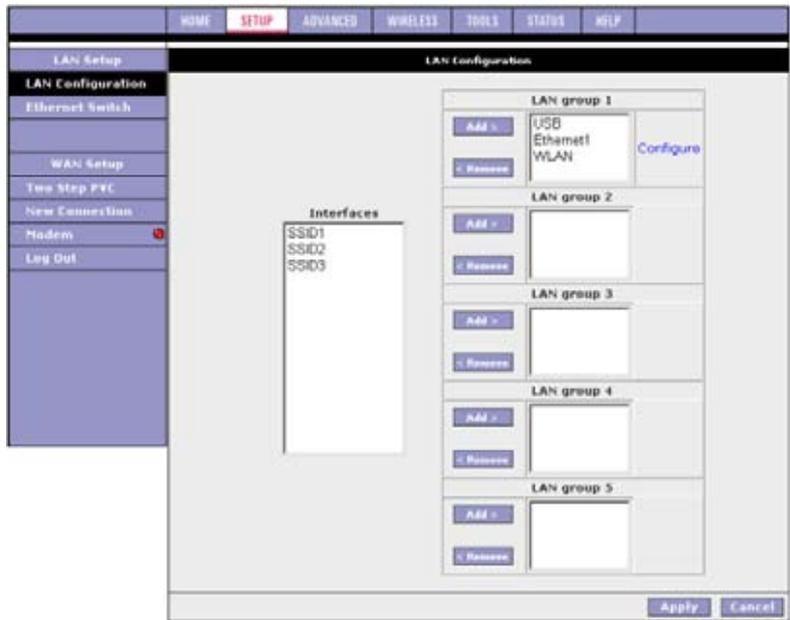
For more information on how to configure multiple SSIDs, refer to "Multiple SSID". The SOHOSpeed performs routing between the LAN group 1 and the WAN connections as shown in figure below.
