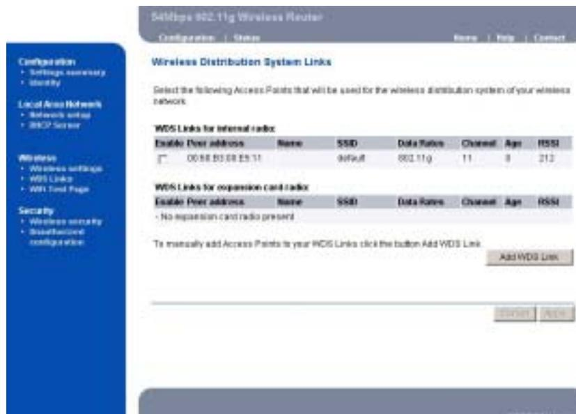
Enter the MAC address of another AP you wirelessly want to connect to into the appropriate field either by clicking **Add WDS link** or selecting the peer Access Point that your Access Point finds out. The implementation can be done as below.
