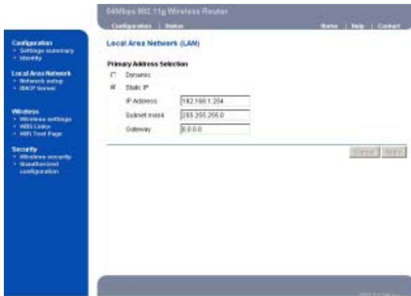
Three selections are provided. If you plan to use any external DHCP server, select **Dynamic**. Otherwise set the LAN address to **Static**. Under the **Static IP**, you have the third choice to turn on the internal DHCP server. First enter the setting on the DHCP server page and enable the default DHCP server. Once DHCP is enabled, you have to make sure the IP address at the **Static IP** settings is in the range of the DHCP server in which the default DHCP server is usually enabled.
