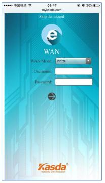
If you have a IP address to connect to the Internet, choose "Static IP" and type in the **IP Address**, **IP Subnet Mask**, **Gateway IP Address** and **DNS Server**.
