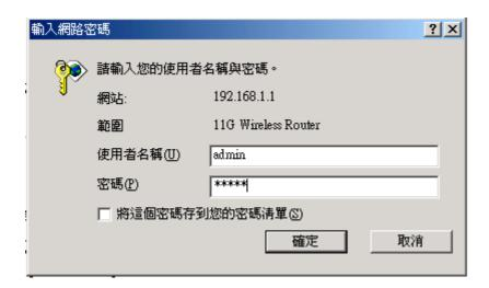
In order to configure the WX-5525G Wireless AP Router, please input the user-name into the **User Name** box. Enter the password into the **Password** box and press the **OK** button. The default username is **admin**, and the default password is **admin**
