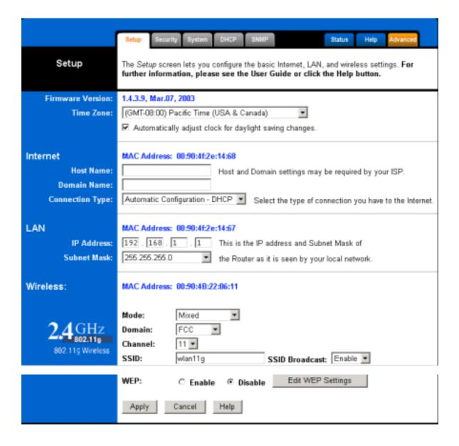
Most users will be able to configure the AP Router and get it working properly using the settings on this screen. Some Internet Service Providers (ISPs) will require that you enter
