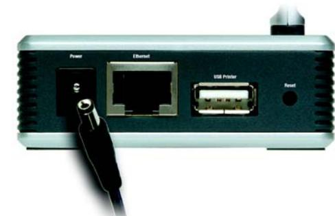
Figure 3-3: Connect to the Power Port
