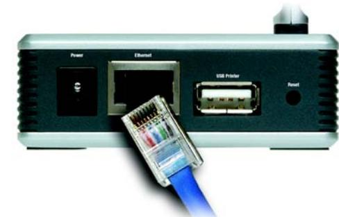
Figure 3-1: Connect to the Ethernet Port
