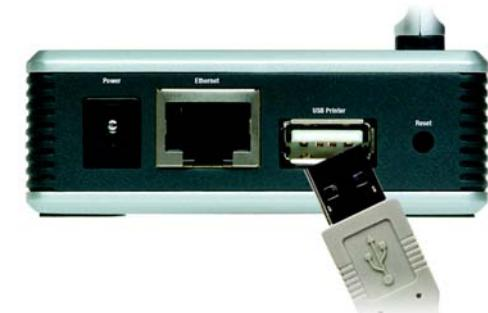
Figure 3-2: Connect to the USB Port
