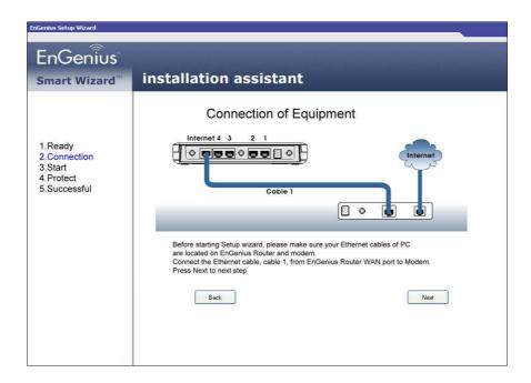
Check the MODEM and ESR-9752 connection. It should be as shown below.
