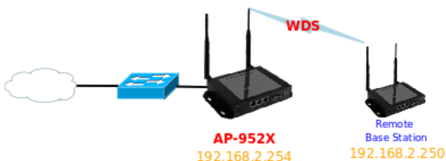
Figure 5-1 Point to Point network Configuration
