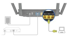
Connect your PC to the router via Wi-Fi or using an additional network cable (not included).
