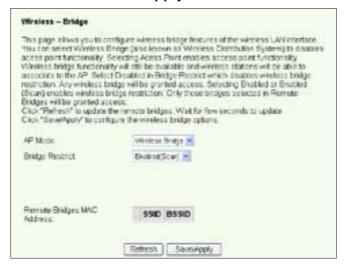
If you cannot find WL-500gD by scanning, set **Bridge Restrict** to **Enable** and input the MAC address of WL-500gD and WL-500gP manually. When finished, click **Save/Apply**. WL-600g WDS setup is complete!
