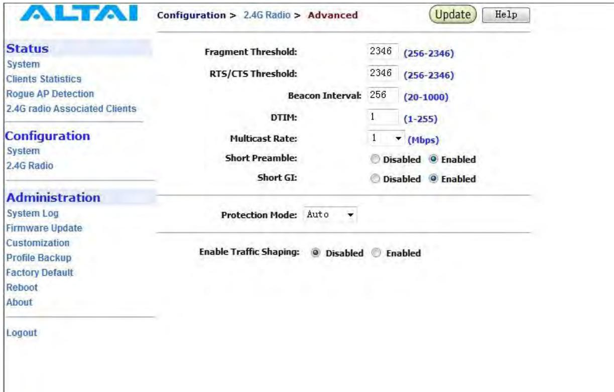
Figure 21 Advanced 2.4GHz Radio Setting
