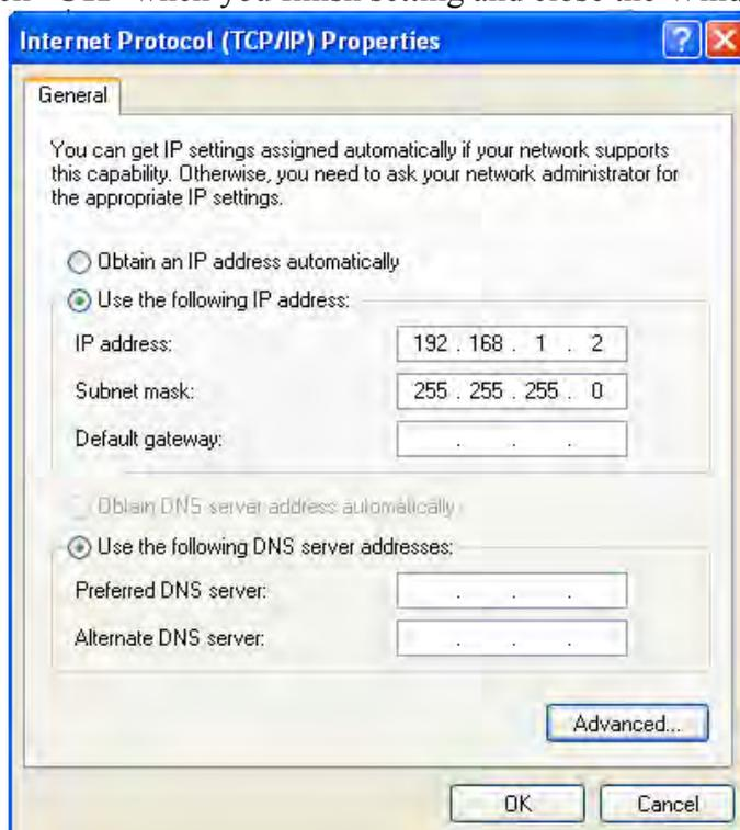
Figure 4 Internet Protocol (TCP/IP) Properties in Windows XP
