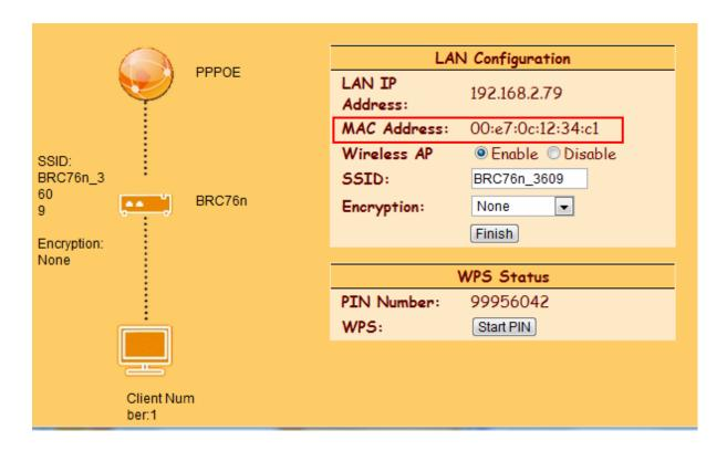
3. Enable WDS function from the page – "WDS Setting", and then fill in the MAC address of Router\_B. Click Apply Changes to save the setting data.
